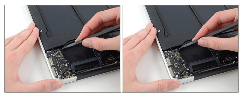
Use the tip of a spudger to carefully flip up the retaining flap on the microphone ribbon cable ZIF socket.
