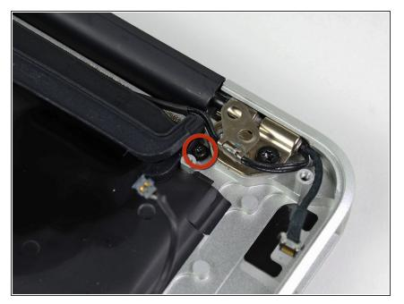
Push the antenna cable retainer away slightly and remove the 3 mm T5 Torx screw securing the end of the heat sink to the upper case.
