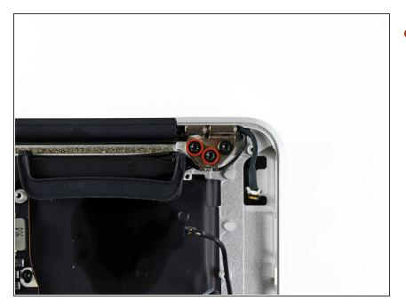
Remove the inner two 4.9 mm T8 Torx screws securing the antenna cable retainer and left clutch hinge to the upper case.
