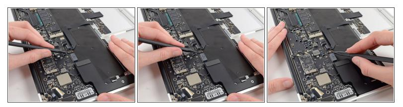
Use the tip of a spudger to flip up the retaining flap on the keyboard backlight ribbon cable ZIF socket.
