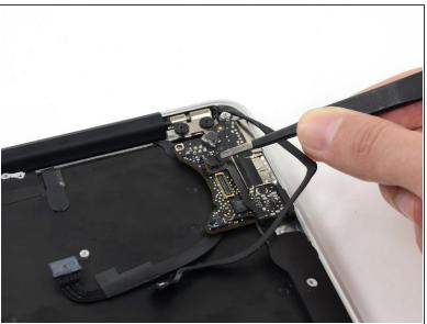
(i) If necessary, use tweezers to remove any tape covering the microphone cable ZIF connector.
