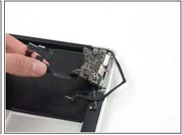
Carefully lift the I/O board by its power cable and pull it away from the edge of the case.
