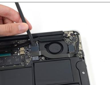
Use the flat end of a spudger to pry the left and right I/O board cable connectors up off their respective sockets on the I/O board.
