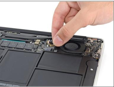
Peel the iSight camera cable up off the adhesive securing it to the fan.
