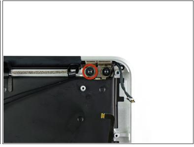
Remove the inner 4.9 mm T8 Torx screw securing each display hinge to the upper case (two screws total).
