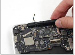
Use the tip of a spudger to de-route the antenna cables from their notches in the logic board.
