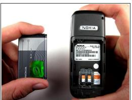
Use a plastic opening tool (or your finger) to gently pry the battery out of the battery slot on the back of the phone.
