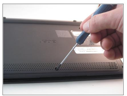
• Locate the 4 mm Phillips #1 screw at the bottom of the back panel. Using the Phillips head screwdriver, remove the screw. Place the screw somewhere it will not be lost. Then remove the back panel by gently sliding it towards the front.
