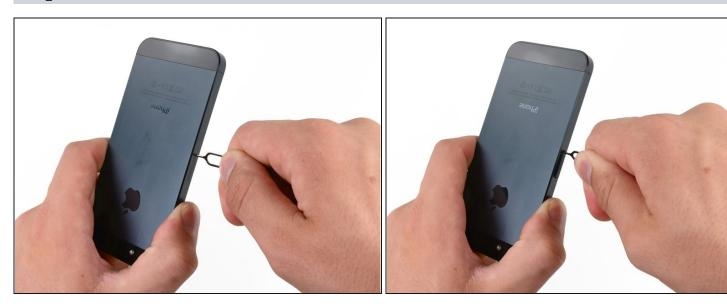
• Use a SIM card eject tool or a paperclip to eject the SIM card and its holder.
