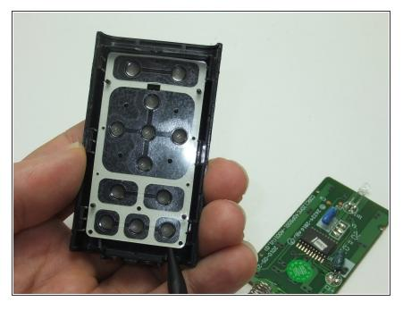
Using either end of the spudger, gently lift and remove the clear keypad backing.
