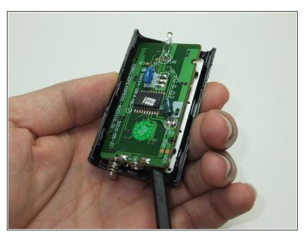
• Gently use the spudger to pry the circuit board loose.
