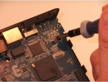
Remove the two Phillips #1 8mm pan-head screws.
