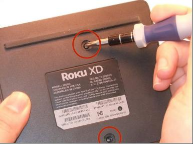
Remove the two Phillips #1 9mm pan-head screws.
