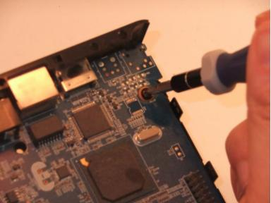
Remove the two Phillips #1 8mm pan-head screws.
