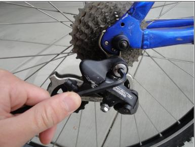
Bolt the derailleur to the mounting tab with an Allen wrench.
