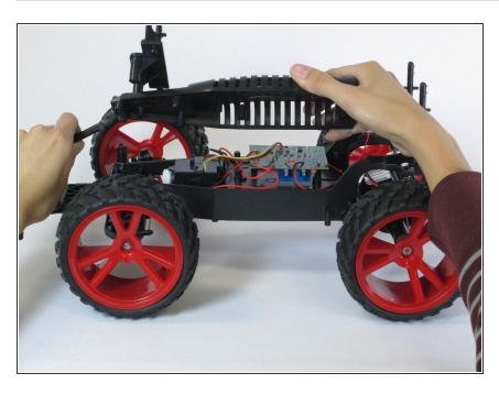
While lifting the part attaching the bumper to the shell of the truck, remove the shell by lifting it upwards and towards the back end of the truck simultaneuously.
