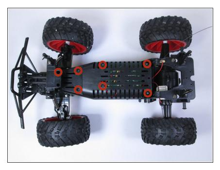
Remove the shell of the truck. Using a Phillips #1 screwdriver, remove the seven 10mm screws highlighted.
