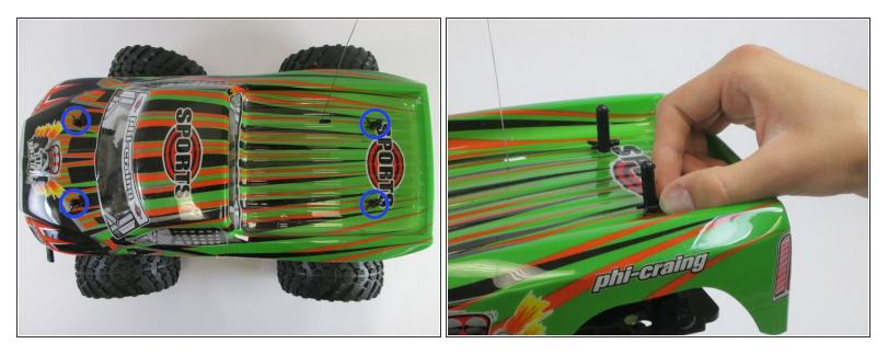
• From the top view, remove each of the four pins that hold the casing in place.
