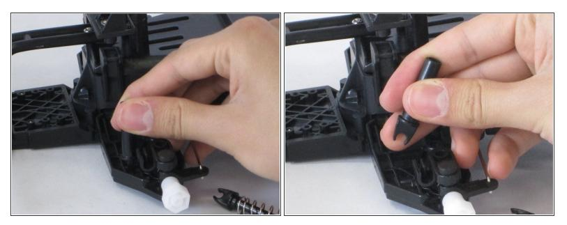
• Pull up the bottom half of the suspension to unclip it.
