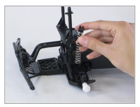
• Remove the top clip along with the spring.
