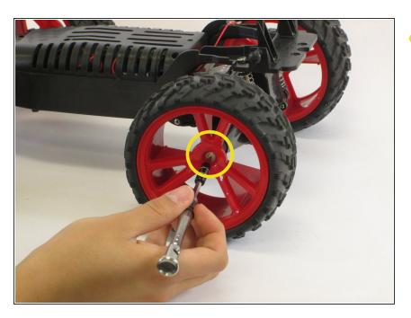
Using a Phillips 1 screwdriver, completely unscrew the 8mm screw located in the center of the wheel.
