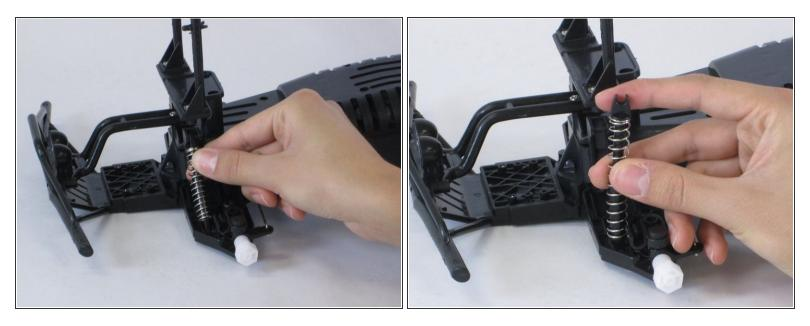
• Pull the top half of the suspension to unclip it.
