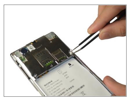
Remove the silicone cover by squeezing it with the tweezers, there is not much pressure needed.
