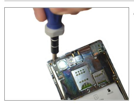
After removing the top left black plate, you will find another 3.13mm screw. Just remove it by using the screwdriver.
