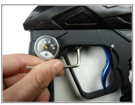
• Remove the front and rear 1" screws on the gun's grip frame using a 3/32" Allen Wrench.
