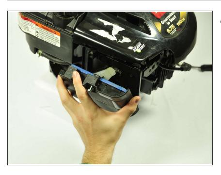
Use your hands to pull the air filter case out of the hinge at the bottom.
