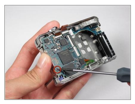
Remove the black screw using a Phillips #00 Screwdriver on the motherboard.
