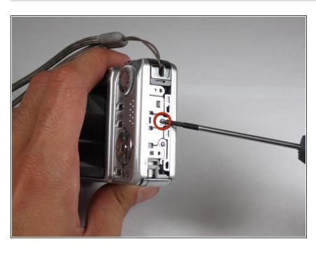
Remove the screw using a Phillips #00 screwdriver on the left side (where the "3x optical zoom" panel use to be).
