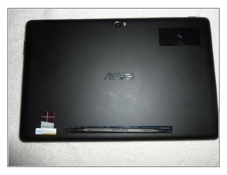
Remove back panel with plastic spudger or other pry tool.
