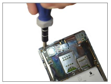
After removing the top left black plate, you will find another 3.13mm screw. Just remove it by using the screwdriver.
