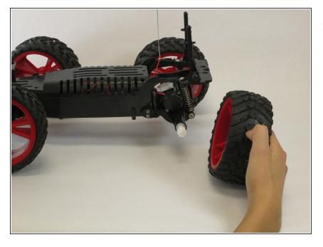
Carefully pull the wheel off of its axle. Repeat for other wheels as necessary.
