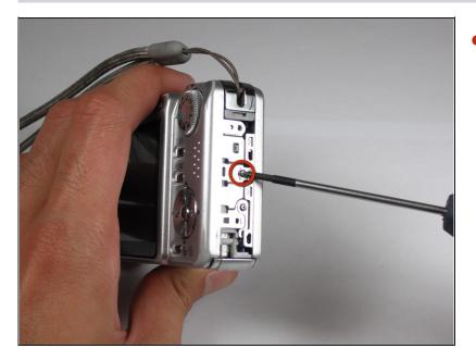
Remove the screw using a Phillips #00 screwdriver on the right side (where the caution panel used to be).
