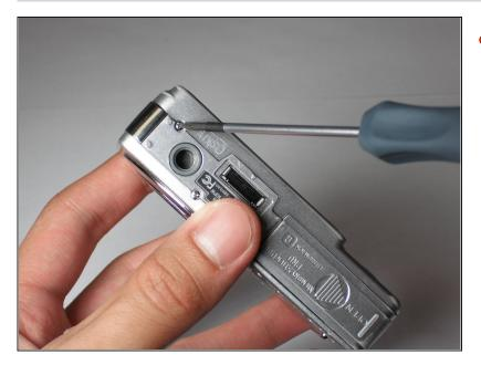
• Remove the screw using the Phillips #00 screwdriver from the bottom of the camera, closest to the back cover.
