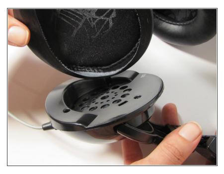
• Continue to detach the cushion from the ear can until it is completely removed.
