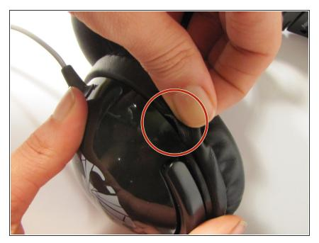
Pinch a spot along the seam of the cushion. Pull up to remove the cushion until the hesh lining is visible.
