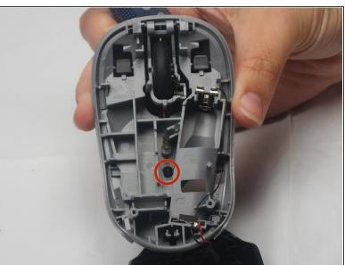
Use your fingernail to carefully remove the two skid stickers from the fat (non-button) end of the bottom of the mouse to reveal two Philips head screws. Remove these, then unclip the bottom cover. Don't get the sticky dusty. Now remove buttons; they're both attached by one 0.5mm Phillips head screw. It is located in the center of the top cover.
