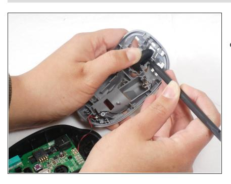
Use the prying tool to remove the scroll wheel. The wheel is held in place by two pegs which stick into the plastic holder. To reassemble your device, follow these instructions in reverse order.
