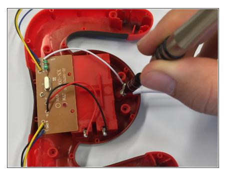
• Remove the 5mm Phillips #0 screw that connects the antennae to the circuit board.
