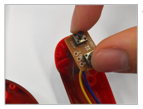
• Remove the two left and right buttons from their insets in the controller.
