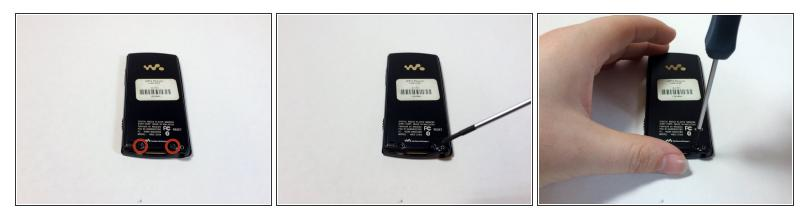
Remove the two black 6.4mm Phillips screws from the back of the device.
