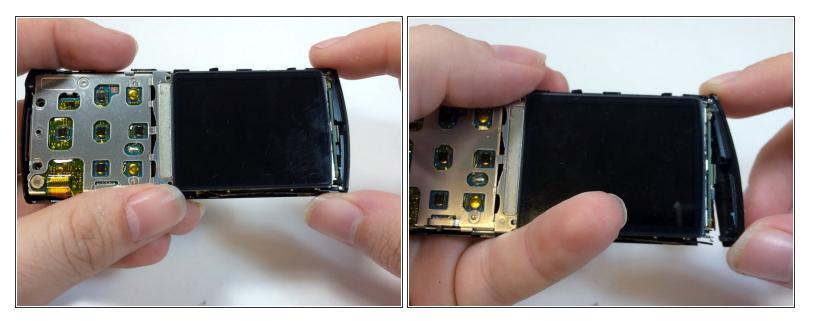
• Carefully pull the top piece away from the device.
