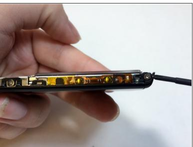
Remove the two 2.8 mm phillips screws located on either side of the device near the top.
