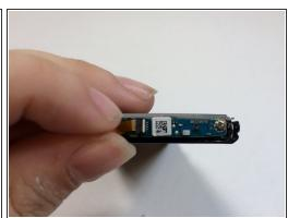
Use the flat end of the spudger to flip up the retaining flap for the bluetooth module.
