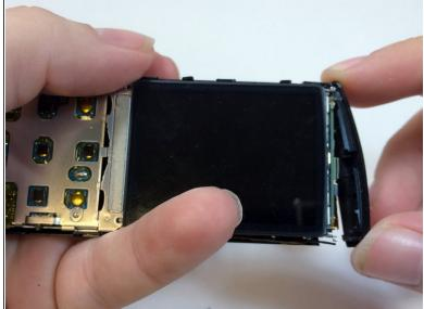
Carefully pull the top piece away from the device.
