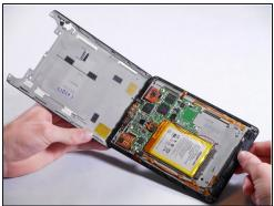
• Once the screws are removed, the back panel can slide off the device.
