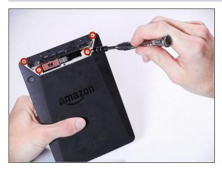
Use an aluminum driver attached with a Phillips head size #00 to remove the four 3mm screws shown in the picture. For reassembly, note that the top two and bottom two screws are different sizes.
