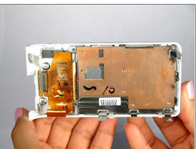
Completely separate the back panel from the camera.
