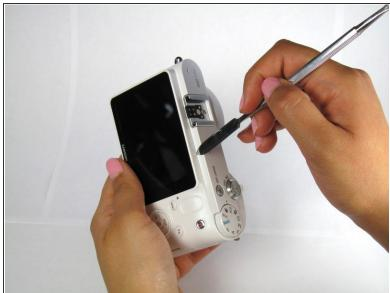
Pry open the back panel using the metal spudger.
