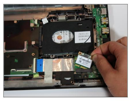
• Slide the component up and out.
