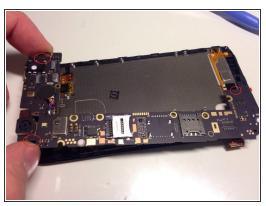
After undoing the flexcables the motherboard can be released (3 spots marked red) and removed.
