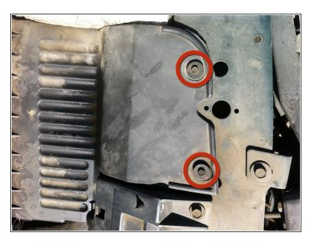
Remove the two 3/16" screws that hold the air filter in place with a 3/16" nut driver.
