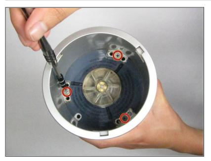
Remove the three 15mm screws with the Philips Head 2 Screwdriver.
