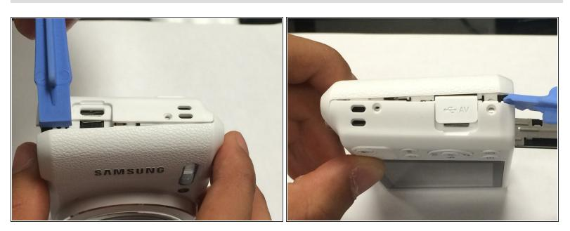
Using the spudger, and plastic opening tool open the casing of camera.
