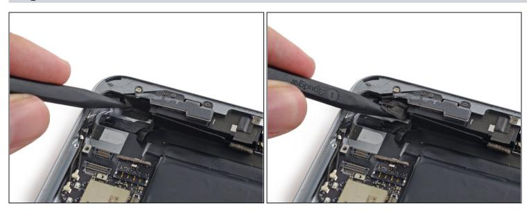
• Use the point of a spudger to lift the antenna cable adhesive up off the rear case.
