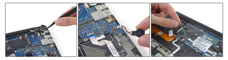
• Tape, cables, and labeled connectors have been the defining characteristics of the XPS 13's guts. There are a lot of components, with a lot of connecting cables, and a lot of tape holding everything down.
