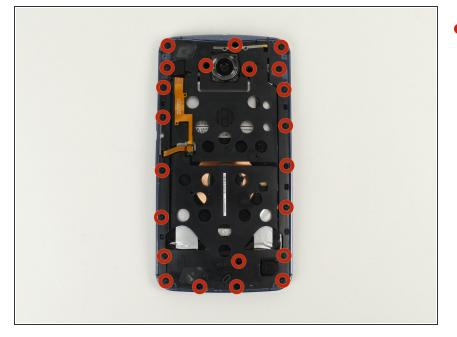
Remove the twenty-two 2.3 mm T3 Torx screws with the T3 Torx Screwdriver.
