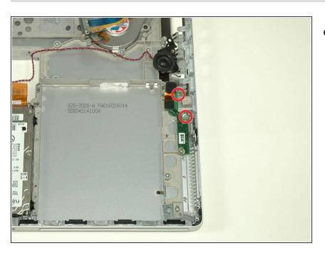
Remove the two silver Phillips screws from the right USB board.
