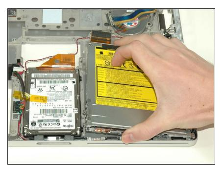
Lift the optical drive out of the computer.
