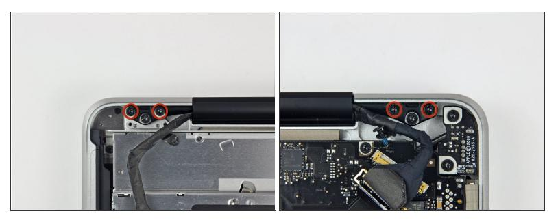
Remove the outer two T6 Torx screws securing both display hinges to the upper case (four screws total).
