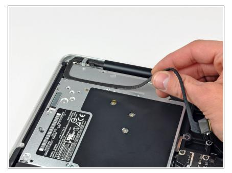
Peel the camera cable off the adhesive securing it to the optical drive.
