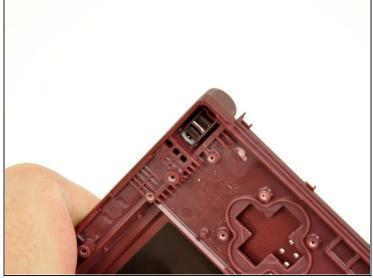
Using a pair of tweezers, remove the LED diffuser bracket and the LED diffuser from the upper case of the DSi XL.
