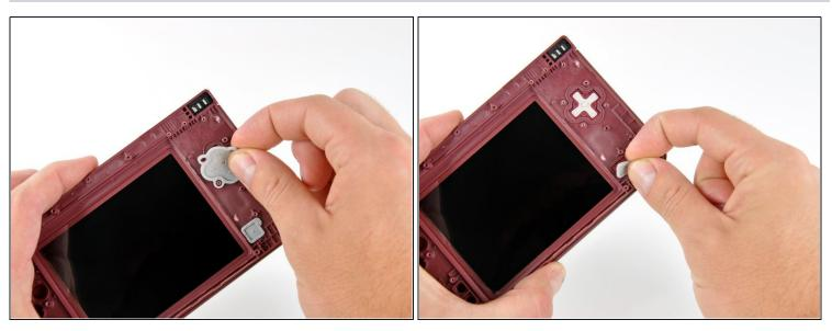
• Peel the rubber button pads off the backside of the D-pad and power button.
