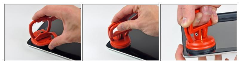
• With the panel sufficiently heated, fasten a heavy-duty suction cup near the upper right corner of the display glass.
