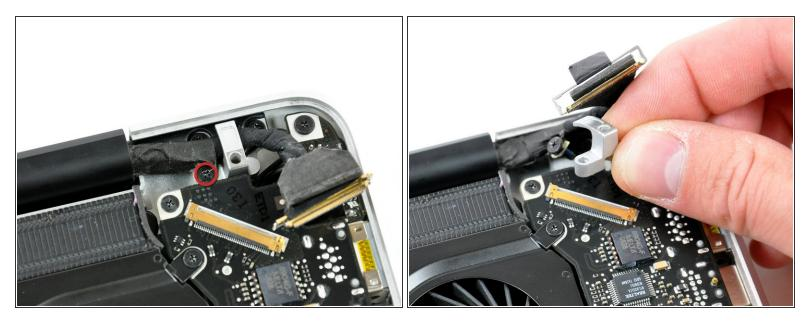
• Remove the 7 mm Phillips screw from the LVDS cable bracket.
