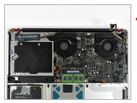
Remove the two outer 6 mm Torx screws securing each side of the display to the upper case (four screws total).
