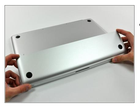
The access door should now be raised enough to lift it up and out of the Unibody.
