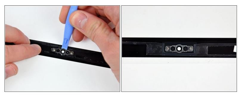
Insert the edge of a plastic opening tool between the display glass and the camera bracket, and run it around the camera bracket to separate it from the display glass.
