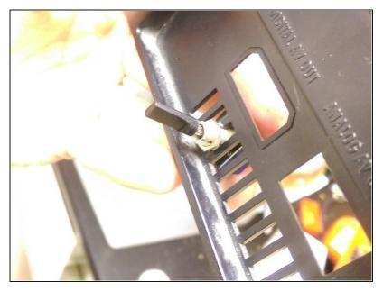
• Insert the switch. In this example, a slot was removed from the vent to allow a larger switch. Make sure your switch is firmly attached and that its position will allow it to fit into the system.
