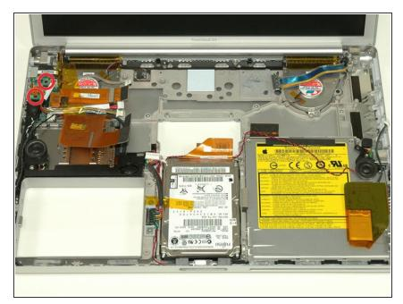
Remove the two 3 mm black Phillips screws from the left ambient light sensor board.
