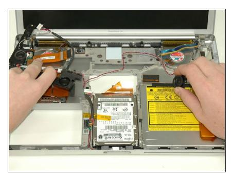
• Lift the speaker assembly (including the right speaker) out of the computer.
