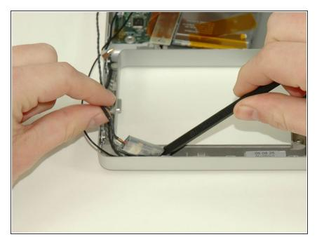
Using a spudger, pry up the Bluetooth board from the cavity in front of the battery compartment.
