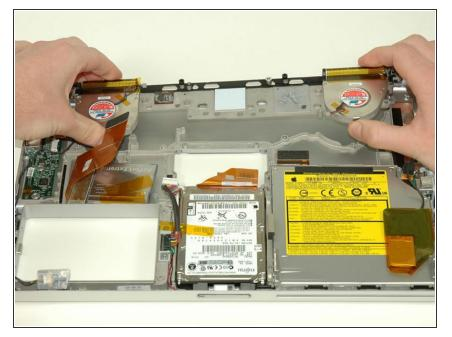
Remove the heat sink from the case, minding the left corner, as it tends to catch in the case (the fans will come out with the heat sink).
