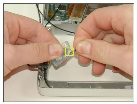
• Disconnect the Bluetooth antenna cable from the Bluetooth board.
