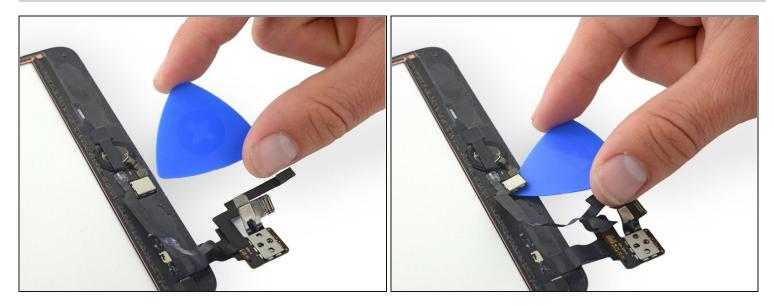
• Use an opening pick to lift the home button control hardware off the back of the front panel.
