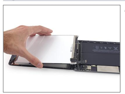
• Lift and remove the LCD from the iPad Mini 3.
