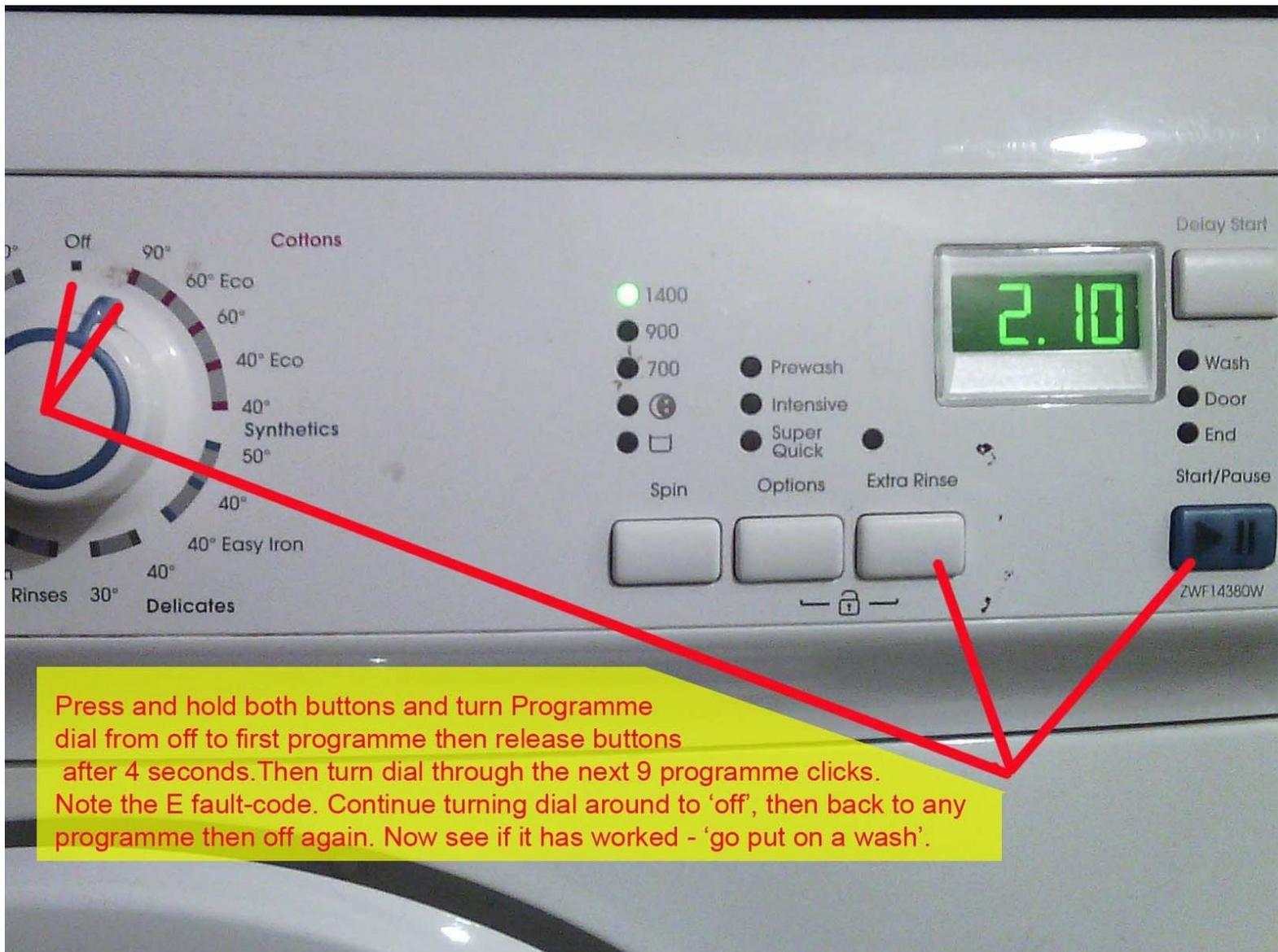
Press and hold both buttons and turn Programme dial from off to first programme then release buttons after 4 seconds. Then turn dial through the next 9 programme clicks. Note the E fault-code. Continue turning dial around to 'off', then back to any programme then off again. Now see if it has worked - 'go put on a wash'.
