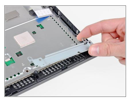
Remove the control board bracket.
