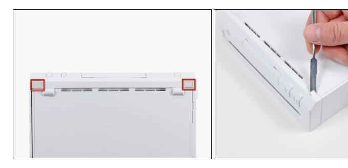
• Use a metal spudger to remove the white plastic screw covers stuck to the lower case near the front of the Wii.
