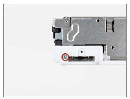
Remove the 8.2 mm Tri-Wing screw that was hidden beneath the battery door.
