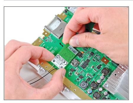
Lift the side of the Wi-Fi board furthest away from the heat sink and lift it out of its socket on the
