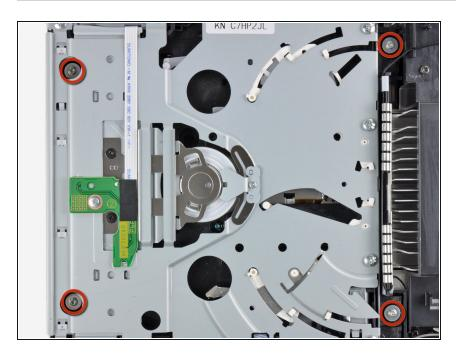
Remove the four 9 mm #1 Phillips screws securing the DVD drive to the bottom panel.
