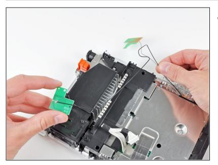
Carefully de-route both antennas from the frame of the Wii and lay them aside.
