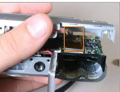
The back half (the half with the screen on it) should now be separate from the rest of the camera, but still attached by the ribbon.
