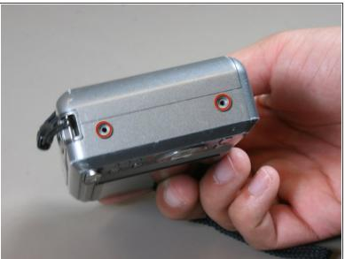
Unscrew and remove the two screws from the right side of the camera.
