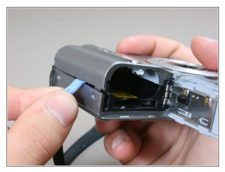
Use a spudger to gently separate the two halves of the camera's outer casing.
