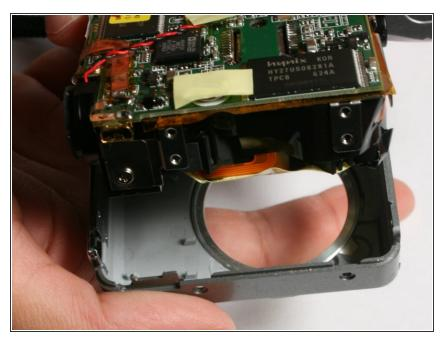
Pull the front half off of the logic board.
