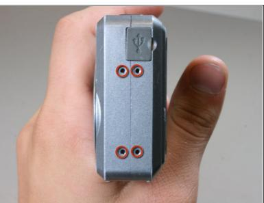
Unscrew and remove the four screws from the left side of the camera (from the screen's view)
