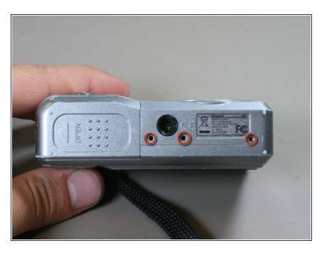
Unscrew and remove the three screws from the bottom of the camera
