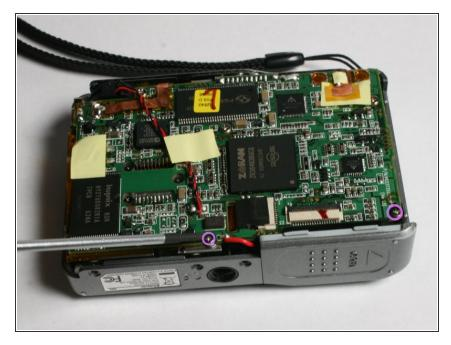
Unscrew and remove two screws from the logic board.
