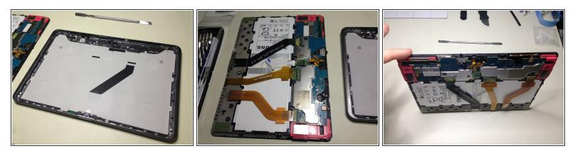
• Once the clips have been released, the front of the device should lift away.
