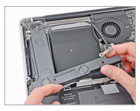
Hold the battery sticker out of the way as you remove the subwoofer & right speaker from the upper case.
