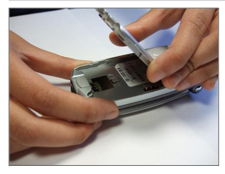
• Lift the battery up from the phone as shown. Replace with a new battery if the old battery has become worn out.
