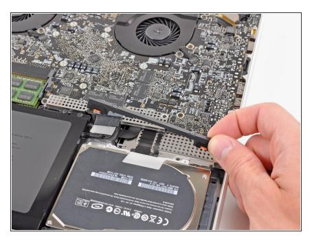
Remove the hard drive bracket from the upper case.
