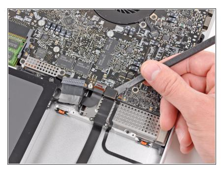
Use the flat end of a spudger to pry the hard drive connector up and out of its socket on the logic board.
